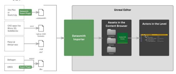
The udatasmith format file can be imported into UE4 by enabling the following plug-ins in U
