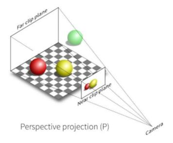
This function modifies the horizontal field of view of the camera, which is the angle bet ween the camera and the leftmost and rightmost midpoints on the top image plane. The defaul t angle is typically 90  $^{\circ}$ .
