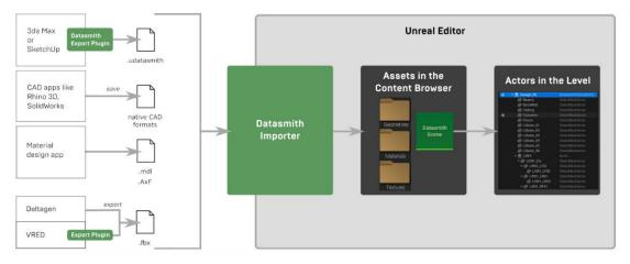
The udatasmith format file can be imported into UE5 by enabling the following plug-ins in UE5.
