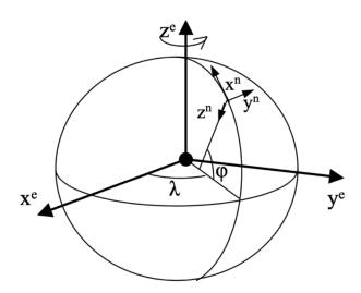
The x-axis points north, the y-axis points east, and the z-axis points to the gr
