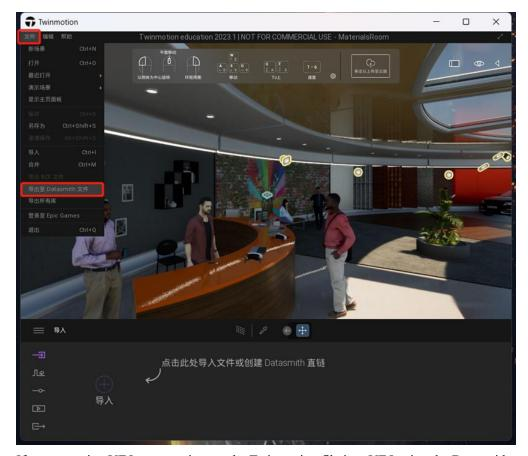
If you are using UE5, you can import the Twinmotion file into UE5 using the Datasmith import method. (The following plug-in "Data Smith Inporter" and "Data Smith Twin motion Content" shall be enabled)
