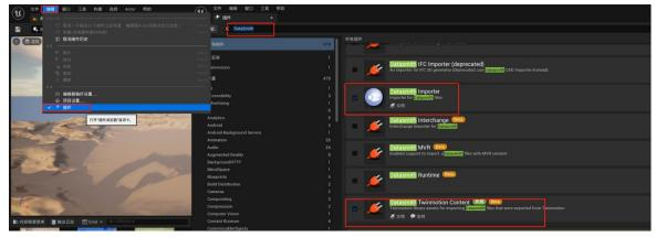
The Data Smith Inporter "will parse the udata Smith file; the Datasmith Twinmotion C ontent" contains various material functions of Twinmotion, which will calculate the ma terial properties of various object surfaces in the scene and assign different material instances.
