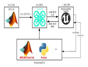
CopterSim calculates the current state of the UAV (mainly position and attitude data) from the motor control data incoming from Pixhawk (or PX4 SITL), and then sends this data to RflySim3D, which applies this data to the corresponding UAV in the scene. So that we can see the state of the UAV more intuitively.
