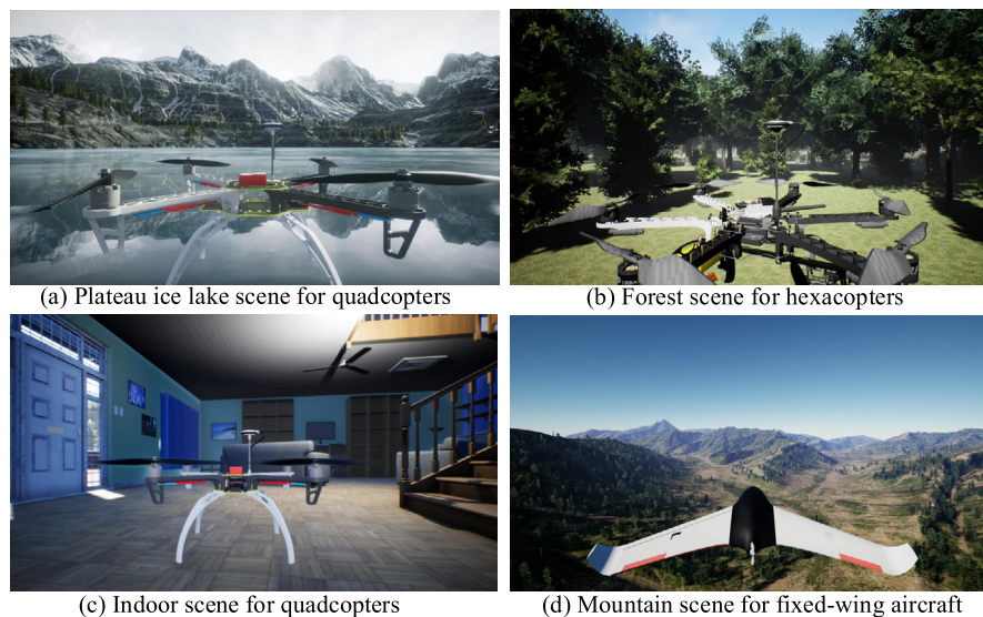
Fig. 11. 3D simulation scenes developed by UE4 for different types of UAVs.
